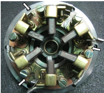
Remove three (3) screws to separate brush holder assembly from the CE frame
