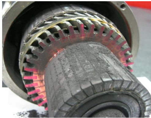
Remove armature to clean brush dust from frame with a nylon brush
